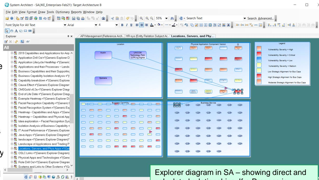
Explorer diagram in SA – showing direct and calculated relationships. If a Process is implemented by an Application instantiated by a Version of the App, draw a line.
